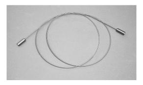
SpeedLoader strings are made with one bullet applied to each end. SpeedLoader strings are made to within .002 of one inch in length, and every string has its own precision length. This precision allows you to change a string and return to perfect tune in seconds.
